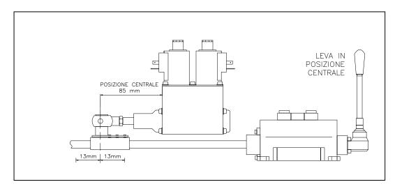
In cases where the reach is not sufficient, it is possible to install an increment kit that brings lever stroke up to a maximum of 40 mm (±20 mm).
