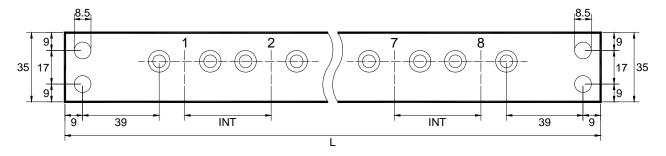
Actuator fixing bar
