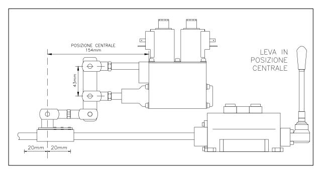
During installation of the Hydra Kit, pay special attention that the actuator and transmission rod are parallel.
