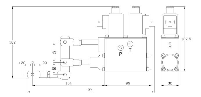
APT 400 Actuator with stroke increment kit
